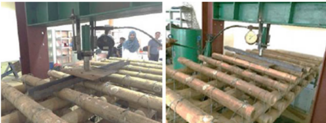
Fig. 7. Loading tests on bamboo mattress.
